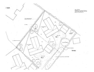
3.2 The dwellings would be c. 14 m wide for 6.3 m back with a 10.5 m projection at the rear that is c. 6.2 m wide. In terms of height, they would be 5.3 m to the eaves and 8 m to the ridge. The double garages each measure c. 6.7 m x 7.2 m, 2.5 m to the eaves 5.3 m to the ridge.
